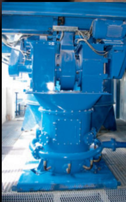
Our newly developed Fluidized-Bed Jet-Mill, based on **microtec** advanced technology, allows for the production of 3 to 150 micron size powders. The mill is primarily used in the production of metal-free and contamination-free products like: Abrasives, Tungsten Carbide, Toner and Pigments. The founder of **microtec** GmbH, Mr. Josef Fischer, has developed an economical closed-loop system for producing "Rare Earth Magnet Powder".
